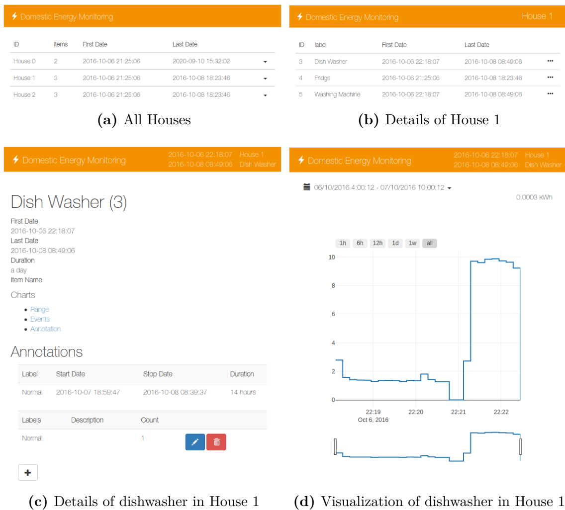
Figure 5.3: Responsive web GUI implemented as part of the central energy server. The tool gives an overview of all collected data including (a) an overview of all houses, (b) detailed view of all appliances in each house, (c) detailed view of an appliance, and (d) a visualization of the collected data.
